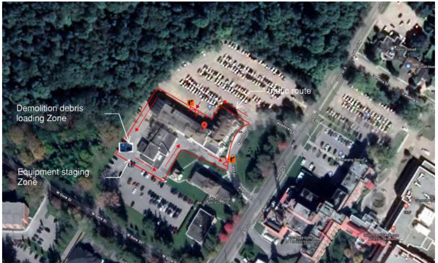
Figure 2: truck staging and loading direction plan
