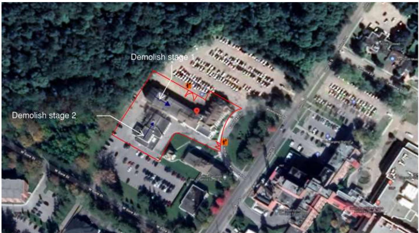
Figure 1: Demolition set-up and overall direction for structural removal, for sequencing and further details on procedures please refer to the Demolition plan
